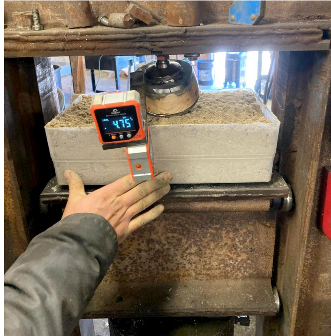
FIGURE 1: The wooden hind foot being readied for the press using two digital levels (see Appendix 1).
