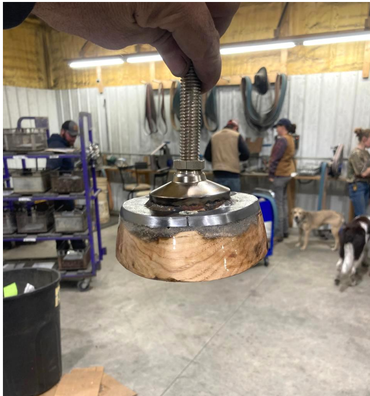
FIGURE 6: The wooden hind foot with a swivel joint attached to the leg side (see Appendix 1).
