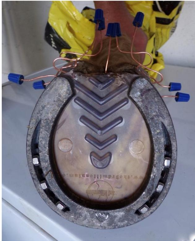
Figure 11: Shod foot with FSP & PU material.
