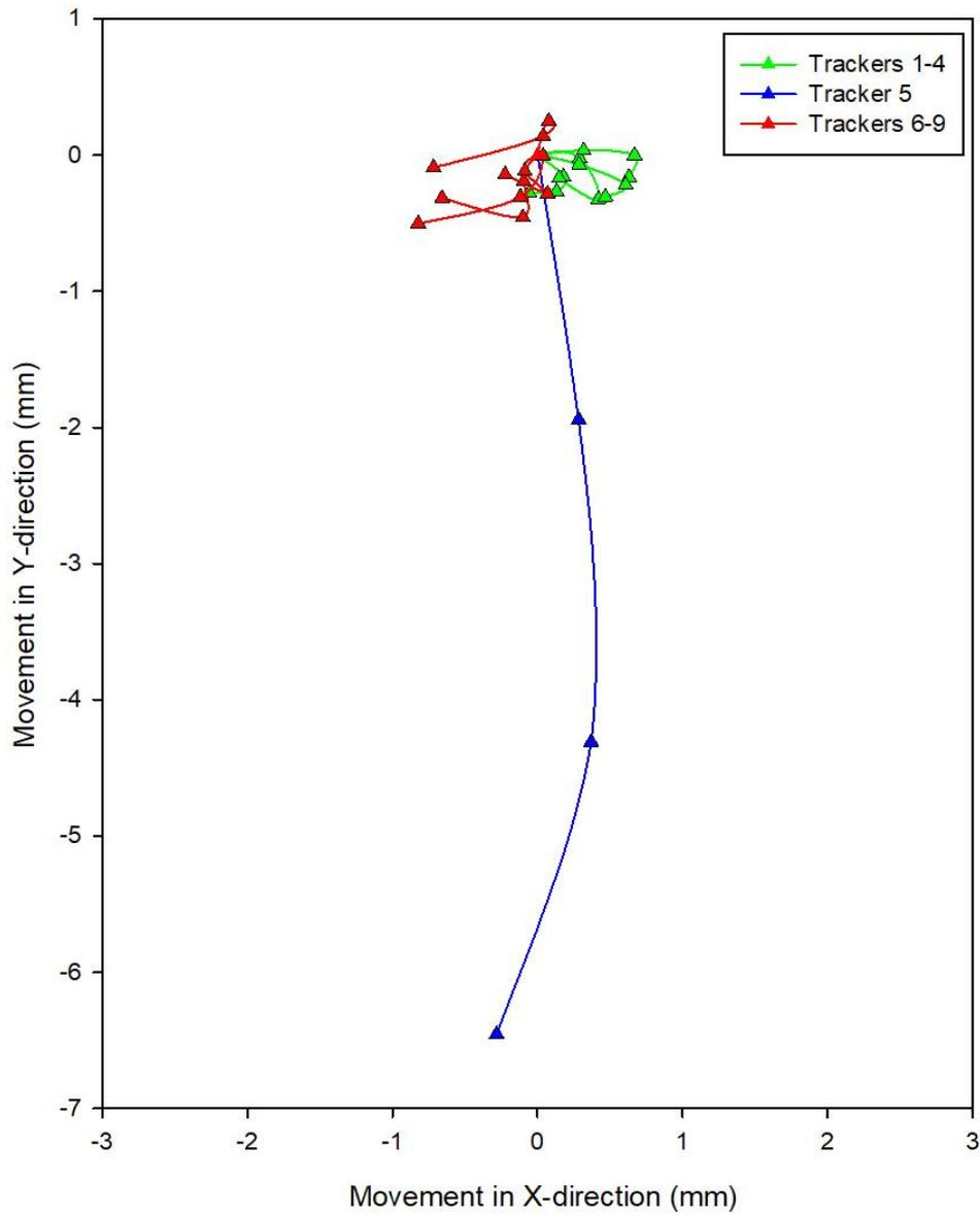
Figure 19: *Movement of trackers 1 through 9, barefoot hoof.*
