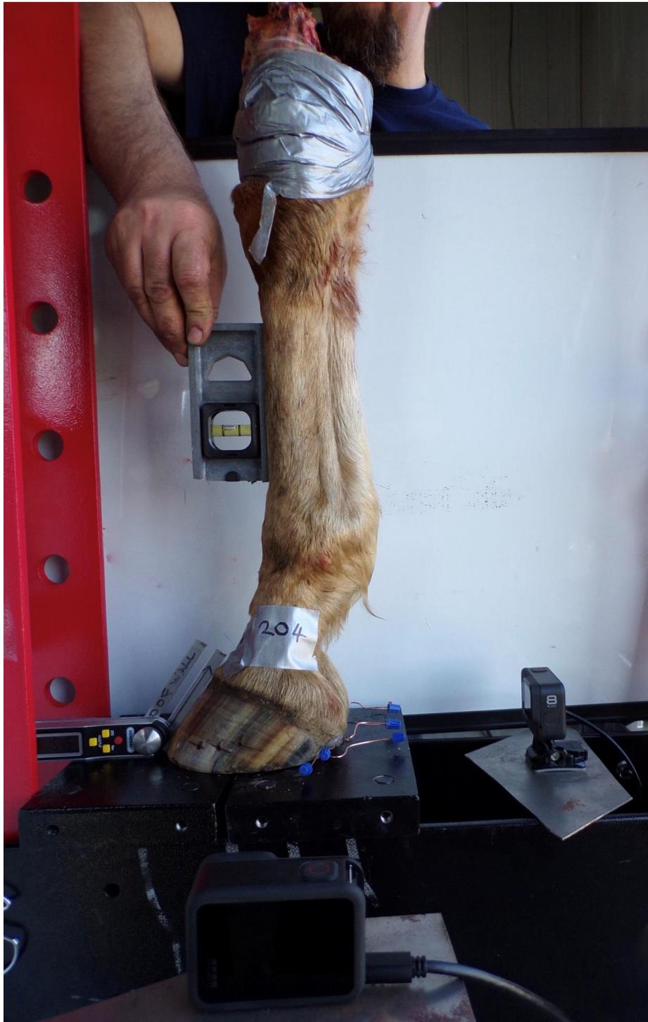
Figure 6: *Pre-limb set up showing camera positions, copper hoof wire locators, IBSL checks & Digital angle protractor (DHWA).*
