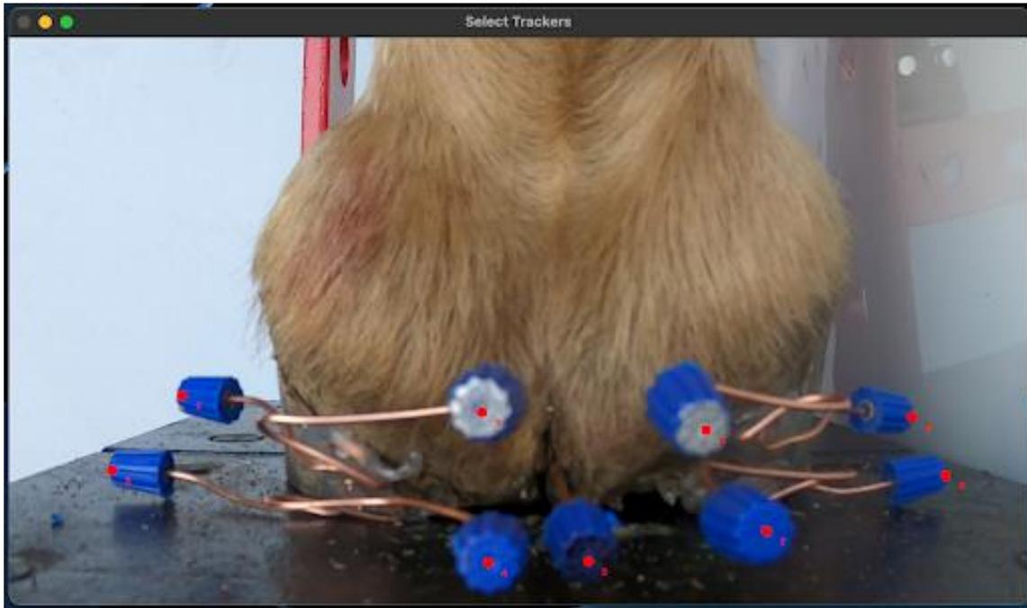
Figure 14. *Visually identified markers through Python numbered 1 to 9 to translate from pixels to millimetres.*
