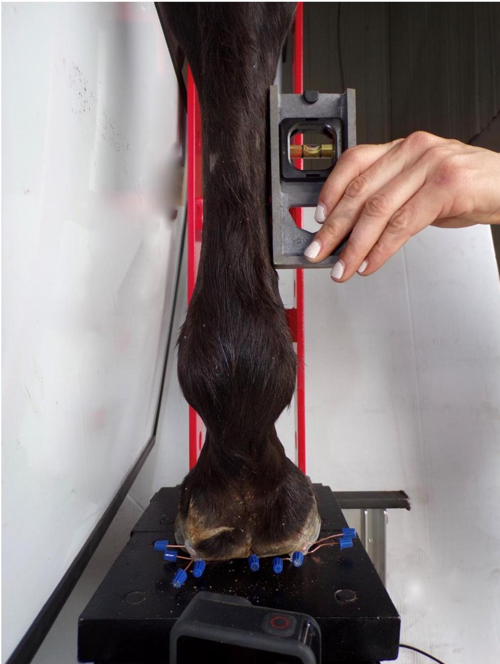
Figure 5: *Pre-limb positional test for IBSL laterally to the mid-cannon upon compression to assert correct vertical & HPA set up.*
