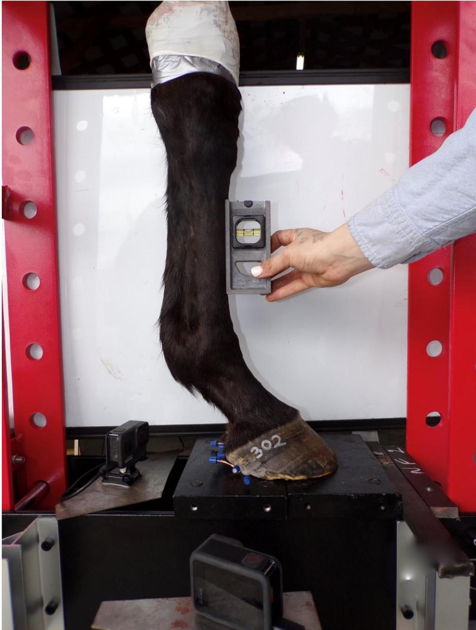
Figure 4: *Pre-limb positional test for I beam spirit level dorsally to the mid-cannon upon compression to assert correct vertical & HPA set up.*
