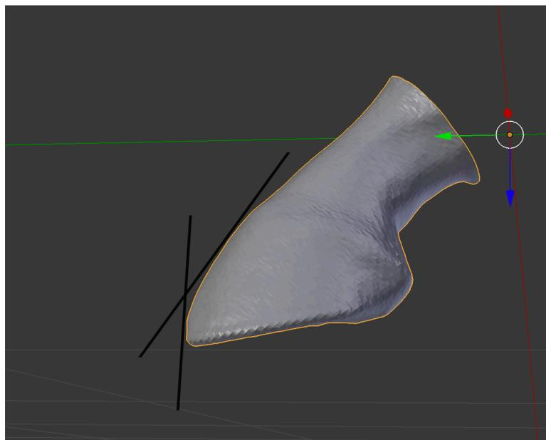
Figure 4.3: Two lines that represent the differing angle that could be taken when measuring the HA on a domes dorsal wall. This ambiguity leaves a large amount of operator interpretation on both CT and 3D analysis and could explain why the WOA were significantly larger than one may expect.
