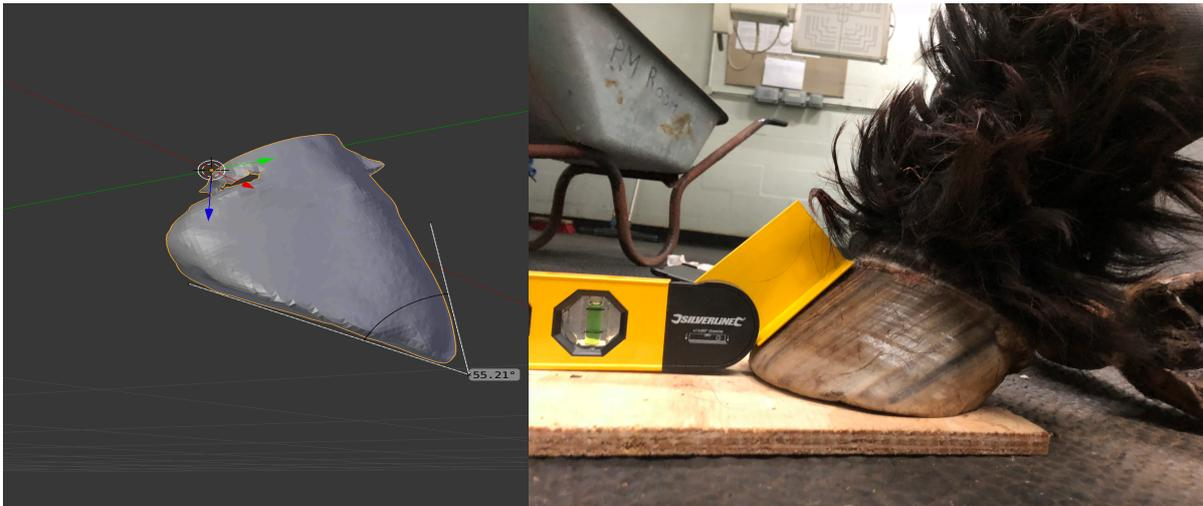
Figure 2.3: HA measurements being collected using 3D data using Blender software (left) and manual measurements with a modified angle gauge (right).
