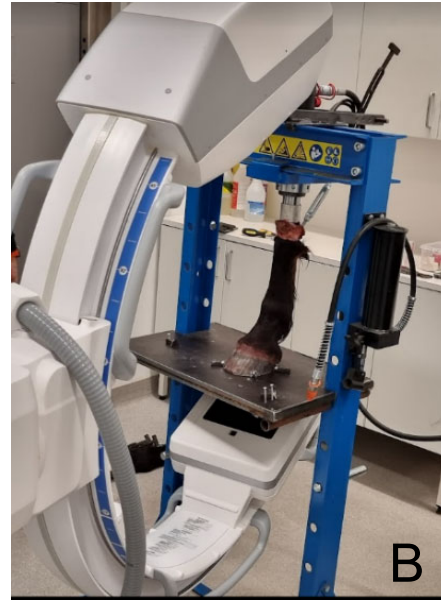
Figure 3: A) two quarter clips and two side clips on a hoof with a Type 3 fracture; B) the set up with a fluoroscope.
