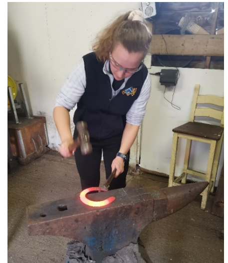
Shaping a shoe on the anvil
