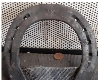
Bar shoe created using a factory shoe and an old rasp
