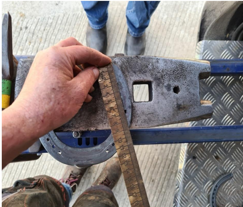
Figure 2: Measuring stud hole placement.
